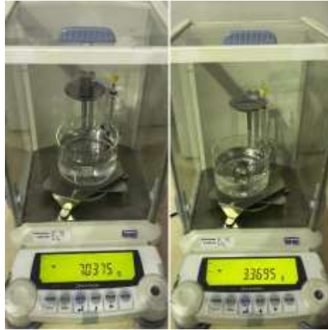
Fig. 2.5. Measurements of weight of the samples in air and water
