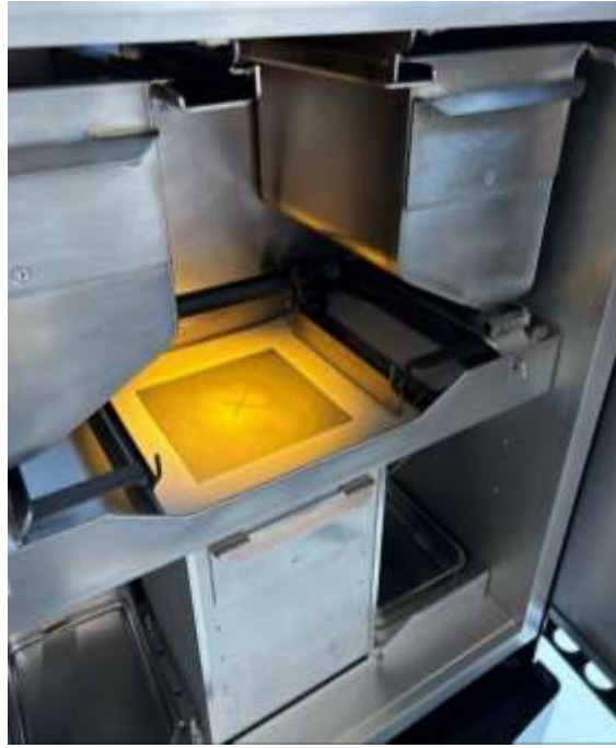
Figure 2.3. Arcam A2X Electron Beam Melting Machine
