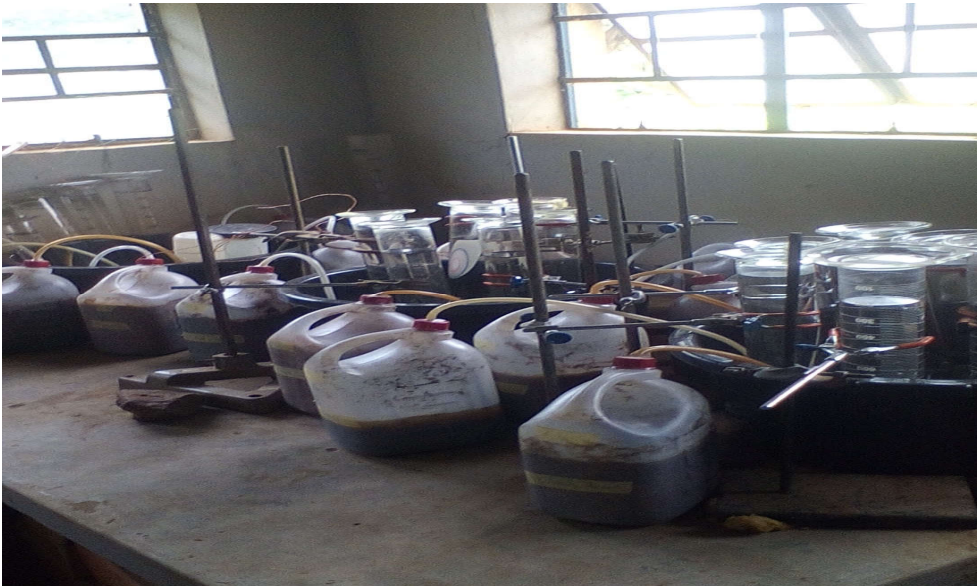
Figure1: Laboratory Set-up for Measurement of Biogas Yield using Downward Displacement of Water
