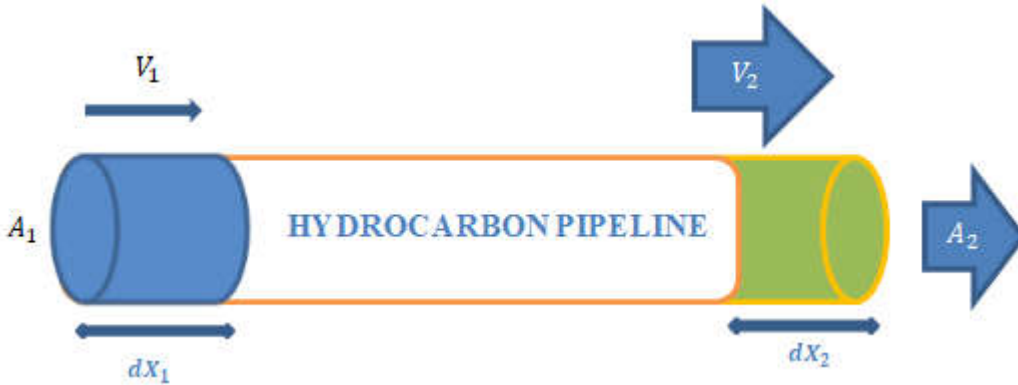
Figure 1: Simple hydrocarbon pipeline flow rate diagram
