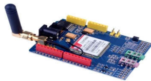
Figure 2. SIMCON SIM900 GSM Module
