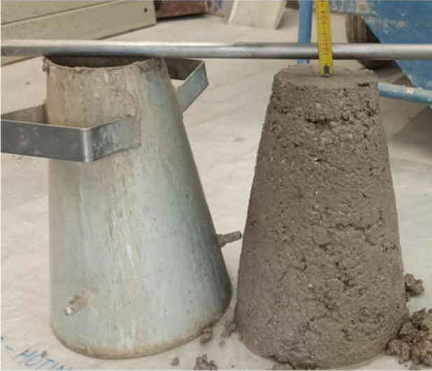
Figure 4. Testing workability by slump method: M-4/8-1
