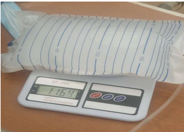
Figure 2: Measurement of Biogas mass in the Urine Drainage Bag
