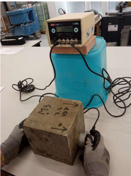
Figure 5. Testing ultrasonic pulse velocity
