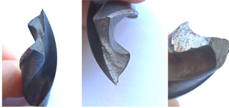
Figure 3. Visual inspection of the fracture surface
