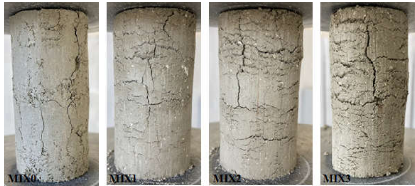
Figure 3. Breakage patterns of the mixture samples after 28 days of curing
